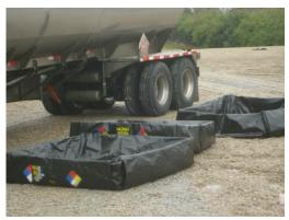
These containment pits can be offloaded just like the saddle tanks themselves by the towing or recovery agency. Containment does not stop the leak or end the incident for responders but it does buy time to establish the things that will terminate the incident.
